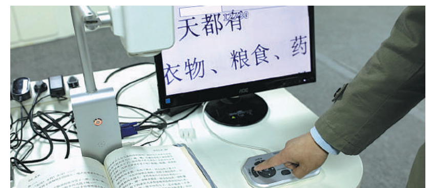
A device to help readers with weak eyesight read. It puts books under a camera that magnifies the text. YANG XIAOHENG / CHINA DAILY
